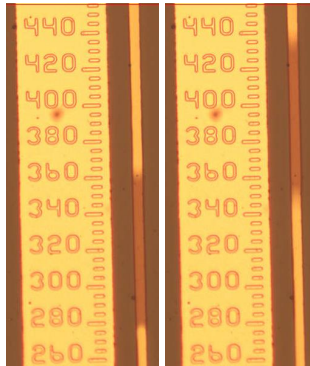
Figure 5.24: Proof of dosing due to gas production. The distance between the two bubbles (light colored) remains \sim 80 \mu\text{m} over a displacement of \sim 75 \mu\text{m} , or a dosing volume of \sim 120 \text{ fL} .
